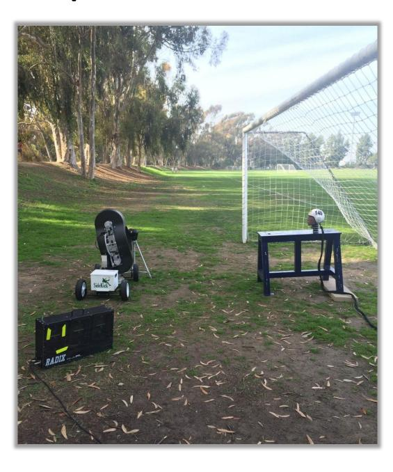
Our testing procedure consisted of launching soccer and water polo balls at an Anthropomorphic Testing Dummy (ATD) head at various speeds and ball pressures, as listed in the table to the right. Six trials were conducted at each speed and each velocity.
